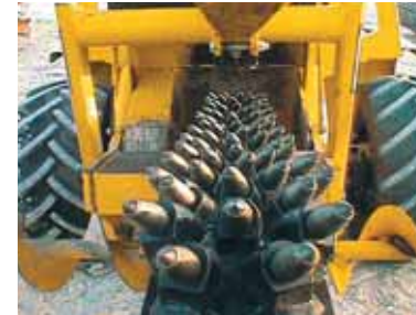
An example of a custom chain used to pulverize Florida coral deposits.
